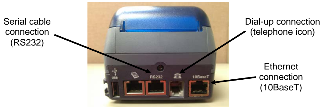
Figure 3 – VeriFone Terminal Connectivity
