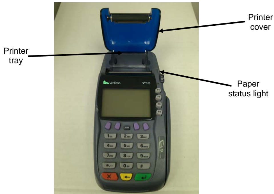
Figure 5 – VeriFone Terminal Front View
