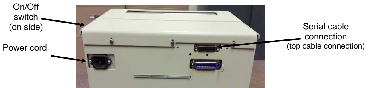
Figure 2 – Money Order Printer Connections
