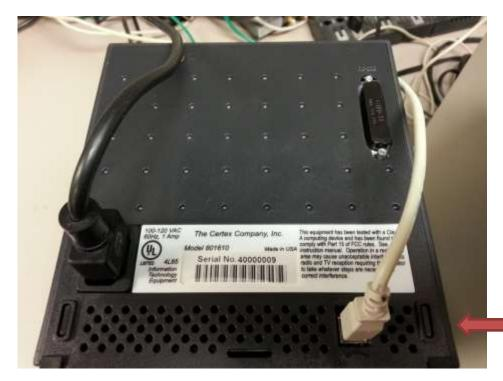
The other end of the cable will need to be attached to your computer by using an available **USB port**.
