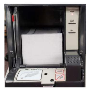
Insert the first Money Order with the **arrows pointing down**. Press the **load button** and push the paper down into the slot. Once the paper is in far enough, the printer will automatically feed the paper to the correct spot. Shut the door and lock it.
