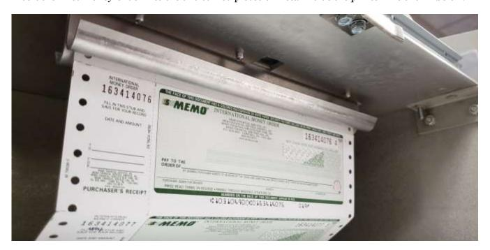
Push the paper up until the holes on the perforated edge touch the black spikes on the roller. Try to align the holes so that they are in line with the black spikes. Turn the silver wheel on the right side of the roller so that the black spikes go into the holes of the paper as shown below. **The black spikes have to be in the same hole on both sides of the paper.**
